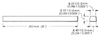
Norm 1—Two Izod specimens may be cut from this bar.
