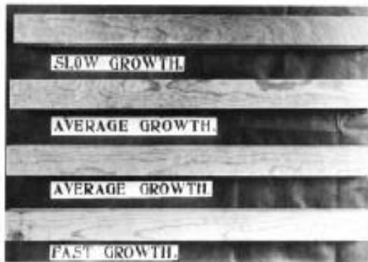
FIG. 2 Tangential Surfaces of Bending Specimens of Different Rates of Growth of Jeffrey Pine 2 by 2-in. (50 by 50 by 760-mm) Specimens
