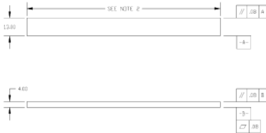
FIG. 4 Standard Flexural Test Specimen Drawing (SI)
