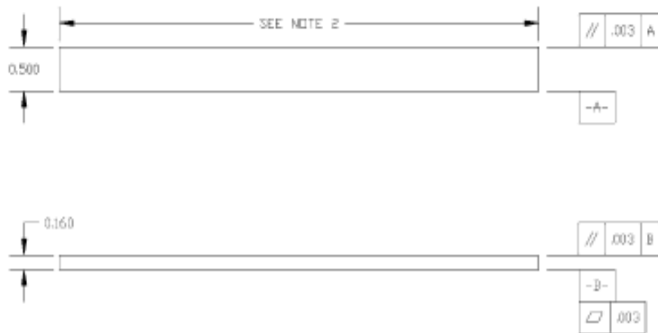
FIG. 5 Standard Flexural Test Specimen Drawing (Inch-Pound)
