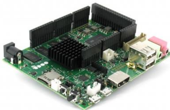
Fig. 2.18 Placa UDOO Dual Basic
