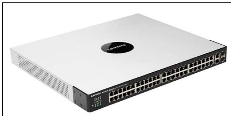
Fig. 21 Switch CISCO 48-Port 10 / 100
