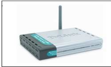
Fig. 23 Access Point D-LINK
