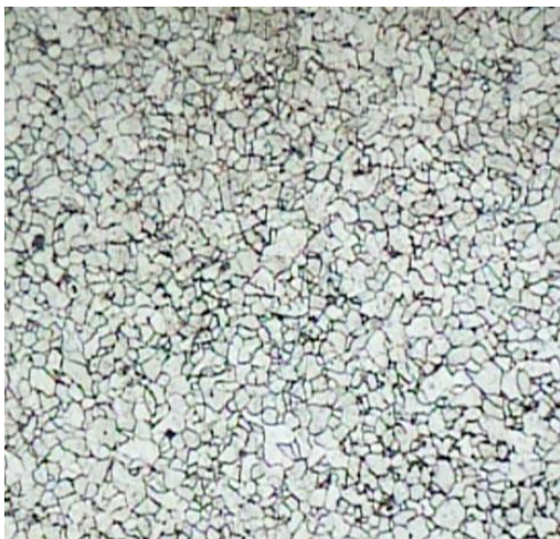
Acero A36 ZAT 100x_Nital4_7s
