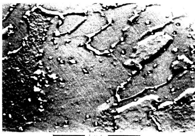
FIG. 6 Example of Replica Microstructure at 5000 \times SEM. Material: See Specification A 335/A 335M, Grade P22. Etchant: 2 % Nital
