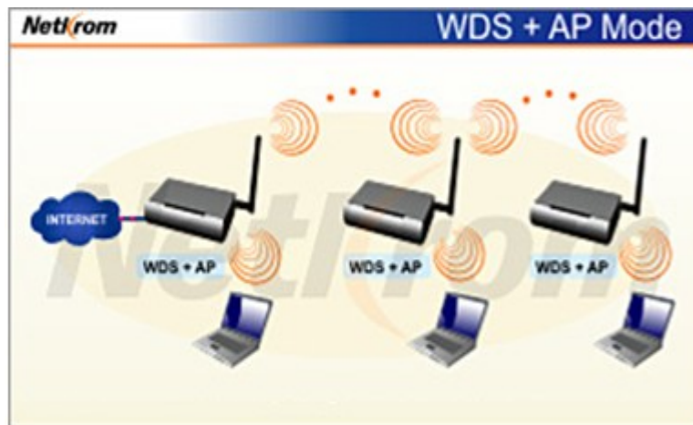
Fig. 5 Modo Access Point + WDS
