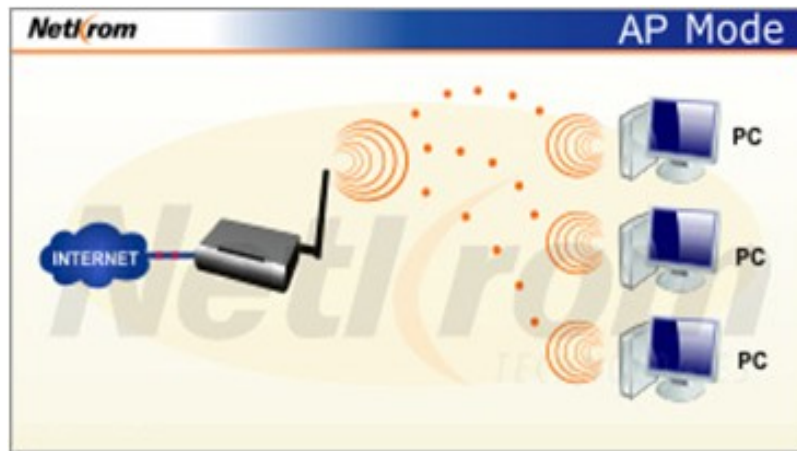
Fig. 2 Access Point en modo Access Point
