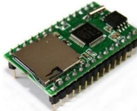
Fig. 4.14 Módulo MP3 WT5001
