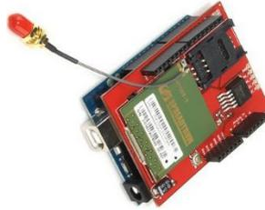
Fig. 4.10 Arduino Cellular Shield - SM5100B
