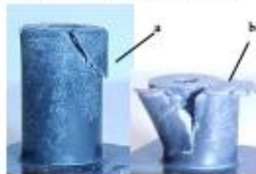
Figure 2. Fatigue failure mode for the boss at compression-compression loading. Agenda: a - shear cleavage along max shear stress plane; b - advanced stage of failure with the break along the knit line.
