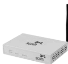
Figura N° 58: 3Com Office Connect Wireless 108Mbps 11g PoE Access Point
