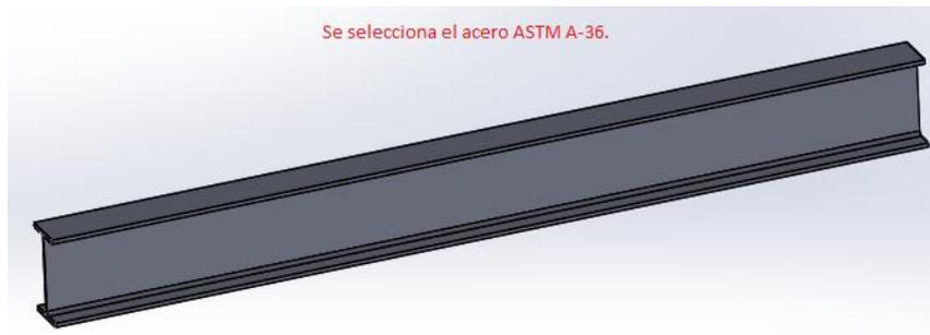
**Figura 6.18:** Viga de acero ASTM A-36.
