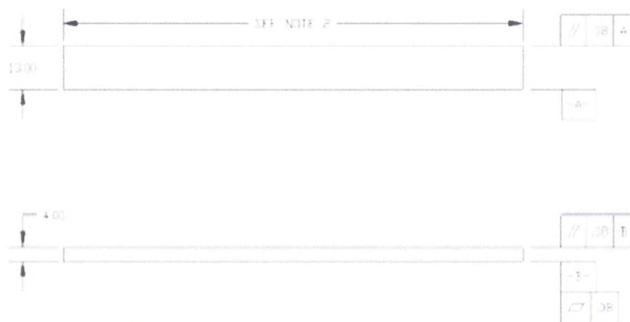
FIG. 4 Standard Flexural Test Specimen Drawing (SI)
