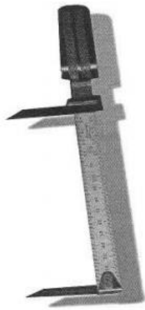
Figura 13. Segmómetro. De: Tilakavati, et al. Limited (ISAK) profiling The International Society for the Advancement of Kinanthropometry (ISAK). Journal of Renal Nutrition and Metabolism, 2018
