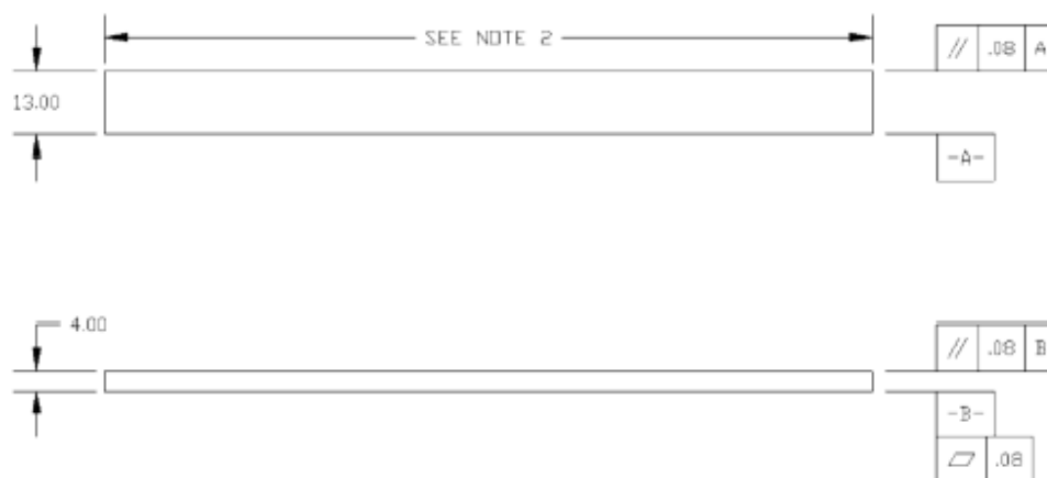
FIG. 4 Standard Flexural Test Specimen Drawing (SI)
