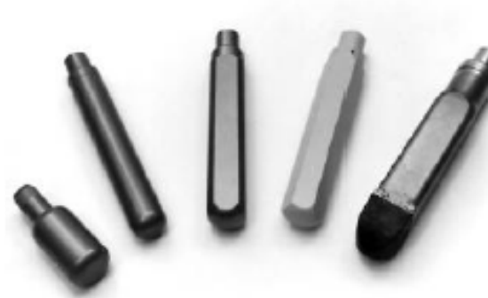
Fig. 5.1.6—Several of the different sizes and shapes of vibrator heads available. From left to right: short head, round head, square head, hexagonal head, and rubber-tipped head
