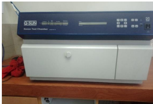
Figura 1.76: Q-SUN Xenon Test Chamber modelo Xe-1-S
