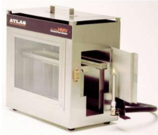
*Figura 6: HMV Horizontal Flame Chamber [9]*
