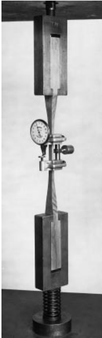
FIG. 29 Tension-Parallel-to-Grain Test Assembly Showing Grips and Use of 2 in. (50-mm) Gage Length Extensometer for Measuring Deformation
