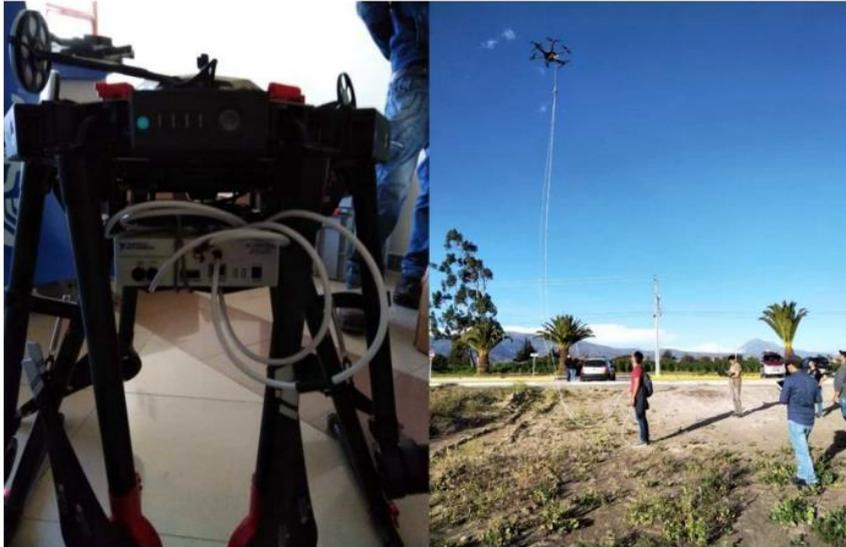
**Fig. 16.** a) USRP and antenna mounted on Matrice 600 drone b) Drone in flight for field performance tests in rural areas.
