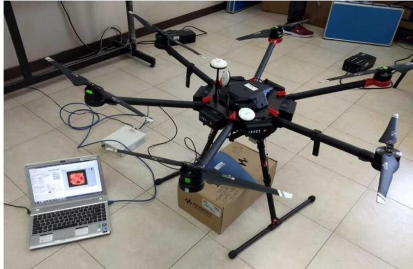
**Fig. 14.** Performance tests in laboratory with logoperiodic antenna and Matrice 600 drone in operation.
