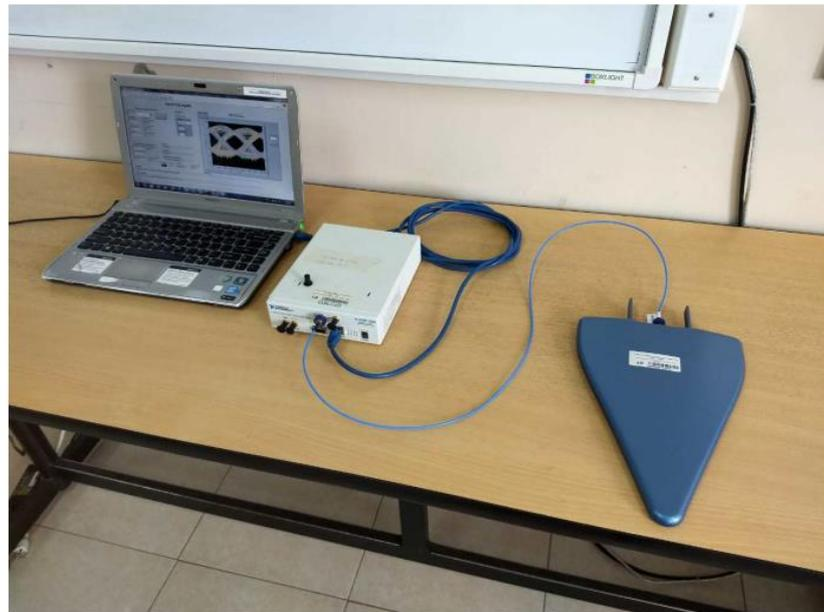
Fig. 12. Performance tests in laboratory with logperiodic antenna.
