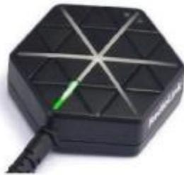
the green LED near antenna will on when SE100 power on
