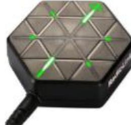
the LED near antenna always on and other LED flicker when SE100 have positioning
