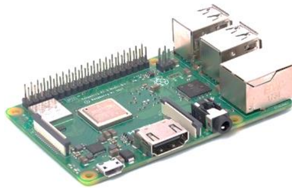
Figura 2. Miniordenador Raspberry Pi 3B.
