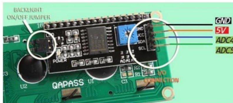
LCD display to Arduino wiring.
