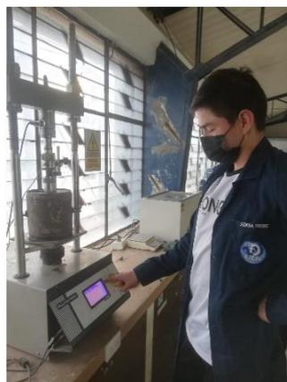
*Figura 30: Ensayo C.B.R.
