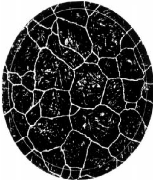
FIG. 4 Example of Austenite Grains in Steel from Plate IV. Grain Size No. 3 at 100X
