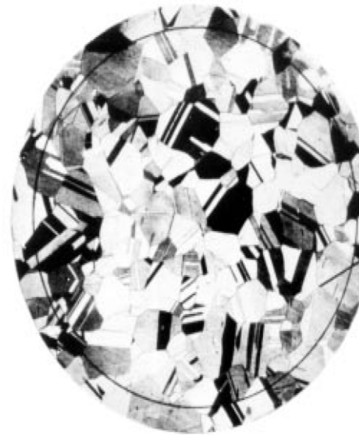
FIG. 3 Example of Twin Grains (Contrast Etch) from Plate III. Grain Size 0.090 mm at 75X
