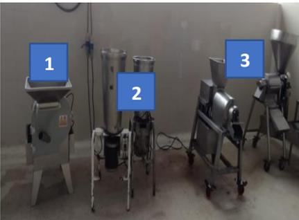
A photograph showing three industrial machines used for fruit processing. Machine 1 is a coconut grater, machine 2 is an industrial blender, and machine 3 is a fruit peeler. Each machine is labeled with a blue square containing a white number. | <p><b>Tipo de Máquina:</b></p> <p>1 rayadora de coco<br/>2 licuadoras industriales<br/>3 despulpadoras de fruta</p> |
