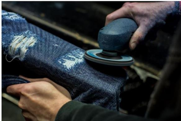
Figura 37: Micro lijado (microsandring)
