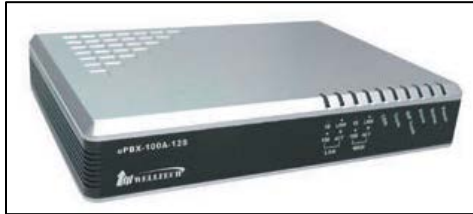
Figura N°6.15. Central IP ePBX100A-128
