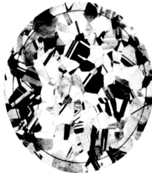
FIG. 3 Example of Twin Grains (Contrast Etch) from Plate III. Grain Size 0.090 mm at 75X
